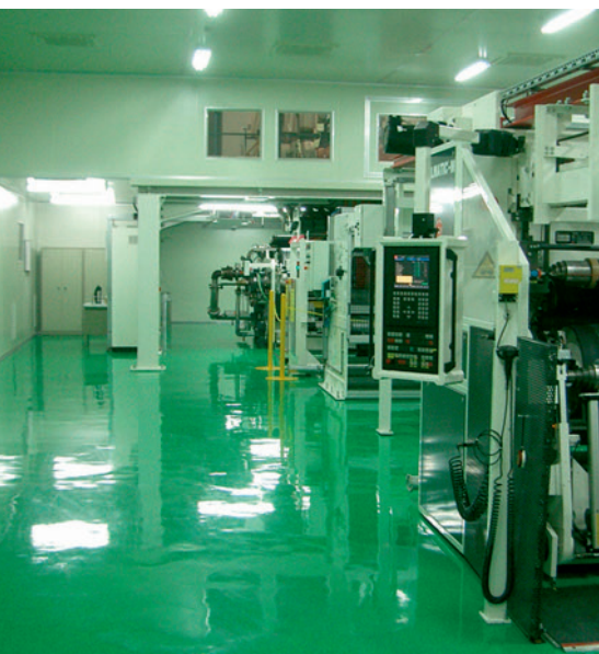
Fig. 7. Filmex cast film line for the production of surface protection films under cleanroom conditions
